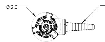
Barb Tip Accepts Tubing I.D from 1/4" to 1/2" Dia.
